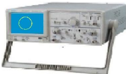
Figure 10: CRO's Output with Non-Faulted Windings
